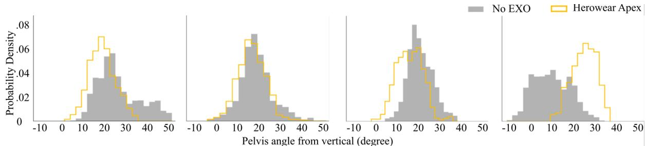
Figure 2. Results for 4 subjects. Changes in movement kinematics, unassisted and while wearing an exoskeleton while dumping a gondola of refuse into a larger cart.
