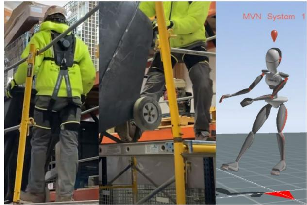
Figure 1. Worker wearing the Hero Wear Apex EXO (Left), pushing then dumping (middle), screen capture from video of motion capture (Right).
