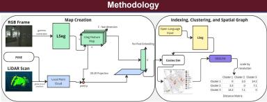
Our method proposes using RGB (gamma correction for brightness), laserscan, and pose input to obtain per-pixel embedding vectors. These embeddings are scored using LSeg for both visual and language input, resulting in a semantic map of a construction site after 3D-2D projection. The resulting classes of objects are then clustered using density-based clustering, allowing spatial relationships to be established between individual instances of each class.
