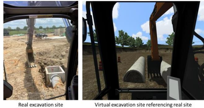
We developed a challenging site scenario that requires participants to dig the soil delicately while avoiding two hazardous buried utilities. In the experiment, participants manipulated the excavator with two joysticks, the control interfaces of the excavator, while observing the movement of the excavator and the surrounding situation in the computer aided virtual environment (CAVE). During the experiment, performance data of operators were automatically collected (Fig. 3).
