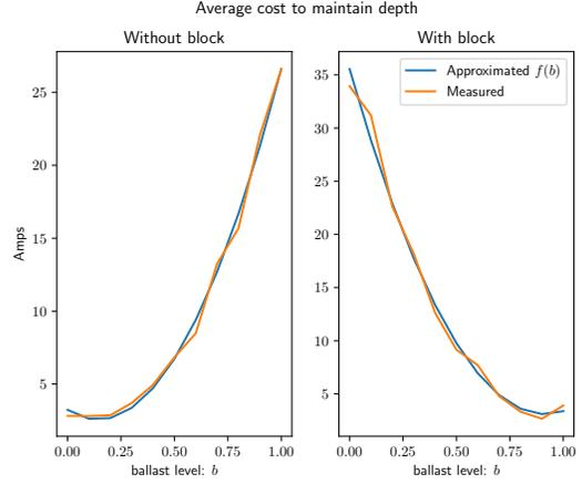
Fig. 5: Calibrated instantaneous cost curves.
