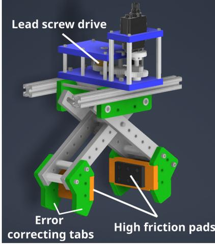
Fig. 3: 3D rendering of 1DOF manipulator.
