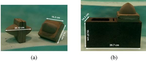
Fig. 4: (a) Cone inserts. (b) Cone insert in block.
