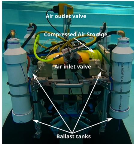
Fig. 2: Active ballasting system.
