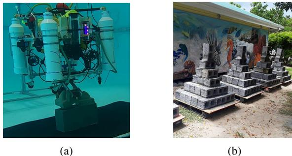
Fig. 1: (a) StoneClaw placing a cone insert. (b) Artificial reefs from the Grande Anse Artificial Reef Project.
