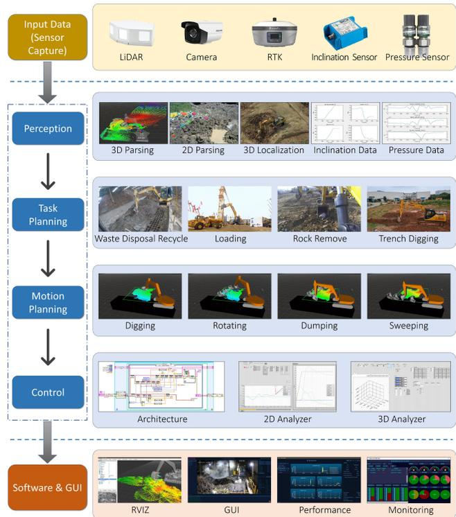
Fig. 1. Overview of Autonomous Excavator System (AES)
