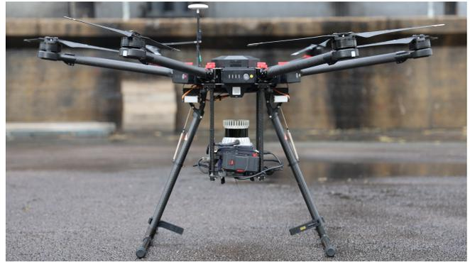
Fig. 2. Photograph of the Osprey aerial platform, a DJI M600 drone with a Frontier sensor payload mounted underneath it.
