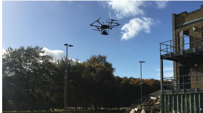
Fig. 1. The Osprey autonomous aerial mapping system surveying a large industrial building.
