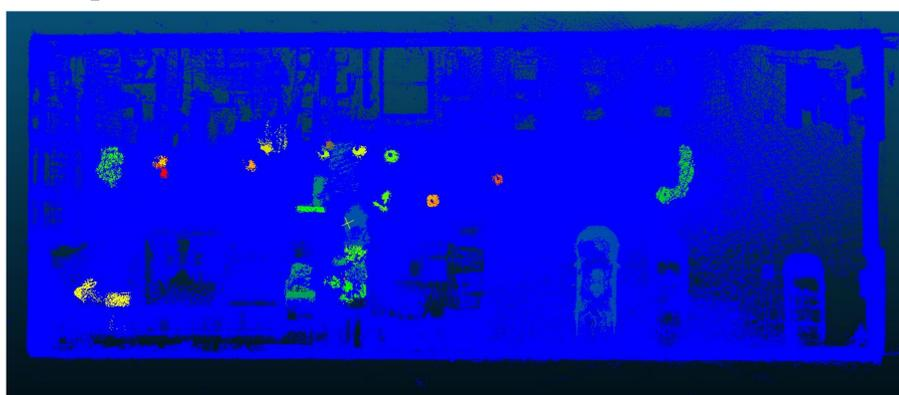
Top down view of multi-mission object based change detection point cloud. Discrete additive and subtractive changed object clusters shown in different colours.
