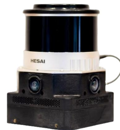
Frontier V7; LiDAR, Camera & IMU in-house sensor suite
