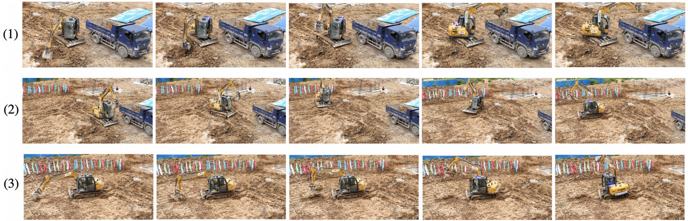
Fig. 4: Snapshots of the experiments. (1) Autonomous truck loading; (2) Terrain navigation; (3) Autonomous trenching.
