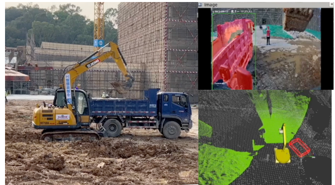
Fig. 5: Autonomous truck loading. During the operation, the 3D truck pose is estimated as shown in the upper-right window, and the task area is designated as a red box as shown in the lower-right window.
