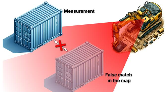
Fig. 1: Semi-static objects treated as static violate the static world assumption and cause mismatches between the map and the measurements. In this example, the map contains a container, which has since been moved away. When the robot returns, an observed container is offset from the one on the map. This offset causes matching errors, especially when the difference in poses is small or other features in the direction of the error are lacking or sparse.
