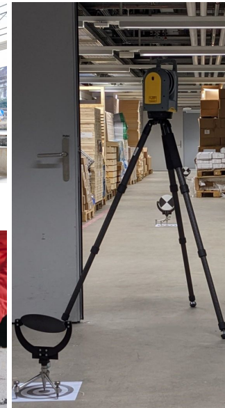
(c) Trimble X7 - Terrestrial Laser Scanner, used for Ground Control Point (GCP) extraction.
