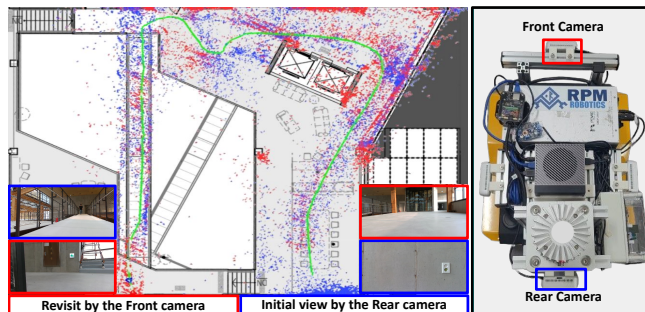
Fig. 1: Odometry and Mapping Results of Our Approach: The visualization features a point cloud delineated by a red boundary, emanating from the frontal camera, juxtaposed with a point cloud encapsulated by a blue boundary, originating from the rear camera. This representation underscores the initial point generation by the rear camera and its subsequent alignment upon the robotic unit’s return.
