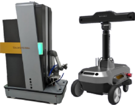
Fig. 7: The employed construction robot cooperated with Transforma Robotics, PTE, Ltd., Singapore, for validation of state estimation accuracy using AM-Align calibrated accelerometer and magnetometer.
