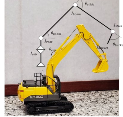
Figure 4. Mechanism and coordination of the simulated excavator
