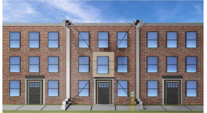
Fig. 1. Conceptual view of a CDPR for retrofitting a residential building using prefabricated panels in a densely populated urban area [4].
