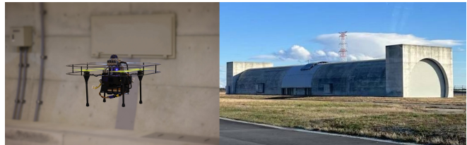
Fig. 1. A UAV performing autonomous inspection in a tunnel-like indoor environment using the proposed method.
