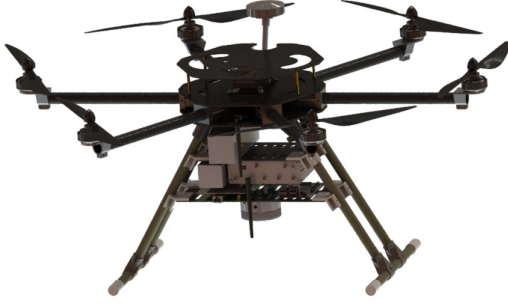
Fig. 3. The CAD drawing of the hexacopter, including the AI subsystem. The carbon-fiber layers situated between the landing gear houses the batteries, RPI, MCU board, 5G router, and camera.
