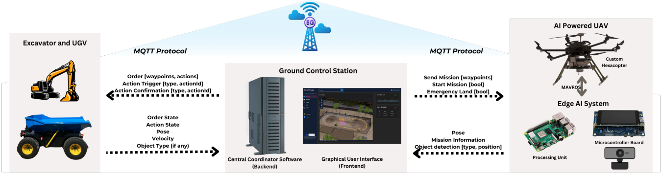
Fig. 2. The overall architecture of the demonstrator is summarized. While the GCS coordinates all the vehicles, communication is facilitated by a 5G mobile base infrastructure. The UAV also contains an Edge-AI subsystem, which is responsible for detecting obstacles in the operational field.
