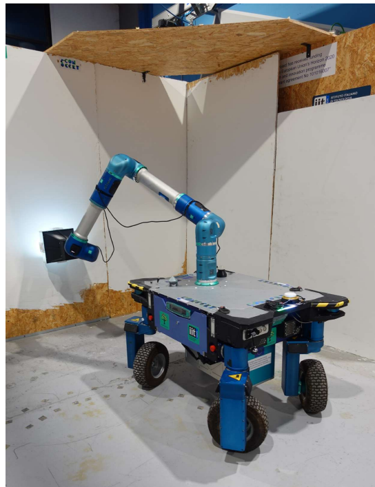
Fig. 1: The CONCERT mobile manipulator autonomously inspecting a putty-coated test wall with the controlled-illumination RGB-D sensing tool.
