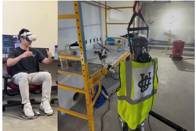
Fig. 1. Humanoid teleoperation for construction task. (Left) An operator controls the robot using a Meta Quest 3 headset and a GYLDR foot controller. (Right) A teleoperated Unitree G1 performs a tool transport task on a job site. It grasps a hand tool (a trowel) from the work surface and carries it toward the destination container (red box).
