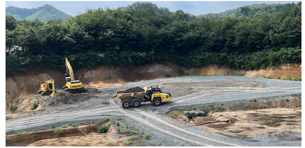
Fig. 2. Autoware-integrated autonomous construction dump truck tested in an off-road environment.
