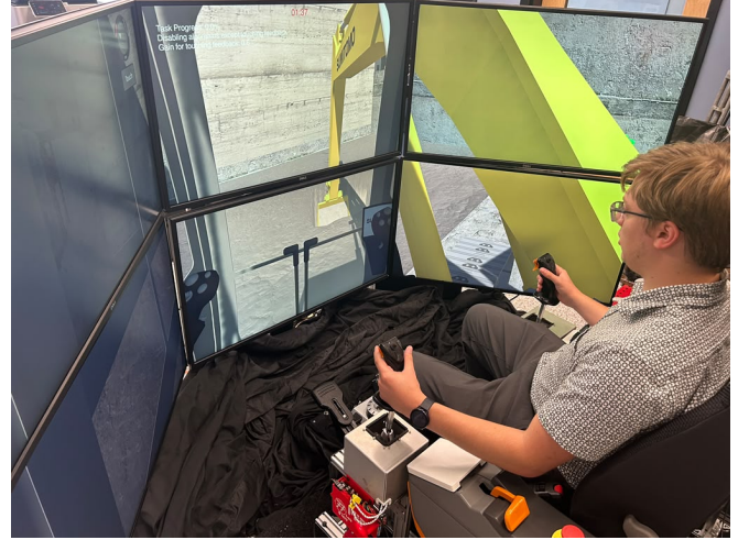
Fig. 1. Virtual excavator operator station used to acquire the joint trajectories evaluated through matched replay.
