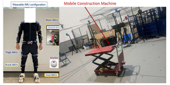
Fig. 3. Experimental setup with the wearable-instrumented worker and representative mobile machine moving in a shared workspace.
