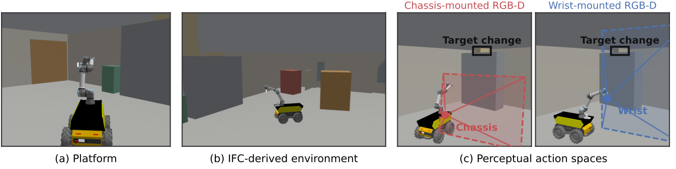
Fig. 1. Simulation study. (a) Husky A300-UR5e platform with identical chassis- and wrist-mounted RGB-D cameras. (b) IFC-derived Hall B with eight injected changes. (c) Evaluated frusta for the same target, which lies outside the chassis-camera frustum but inside the wrist-camera frustum. Each view uses the base yaw that directs its sensor toward the target.
