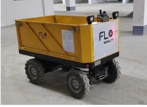
Fig. 1. The custom AMR platform used for multimodal data collection, purpose-built for autonomous navigation in construction environments.
