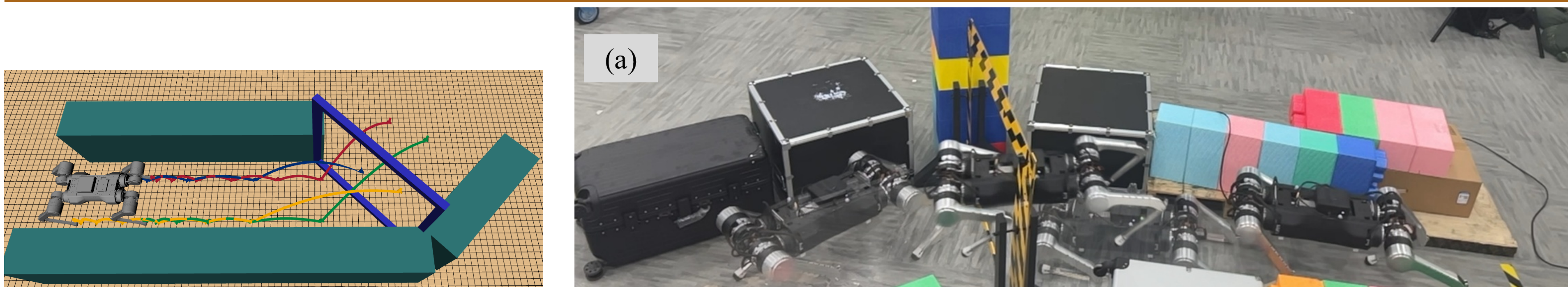
Planning visualization and hardware sequence. Optimized body and foot trajectories define the prescribed maneuver; the multi-pose image shows the corresponding passage through the frame.
