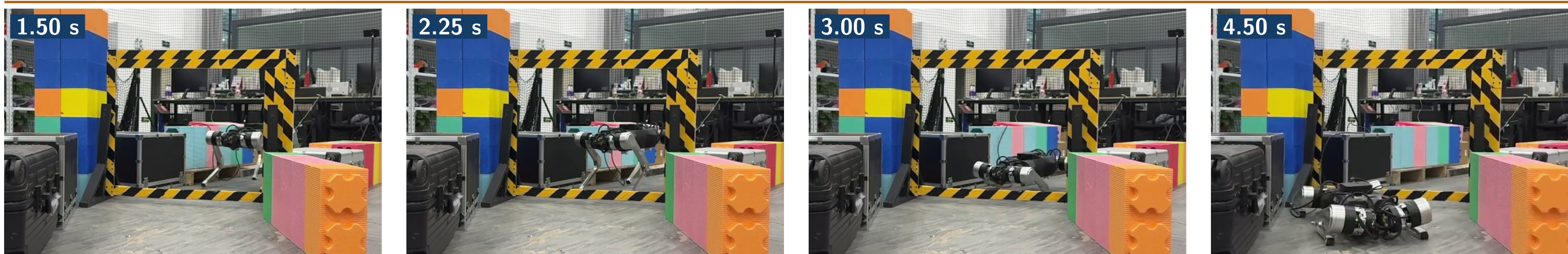
Constrained-opening jump. Selected frames show approach, entry, frame passage, and recovery. Task geometry and the contact sequence are prescribed.
