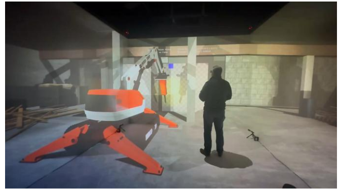
Figure 1. View of the virtual indoor demolition site with the virtual demolition robot and a real human operator.
