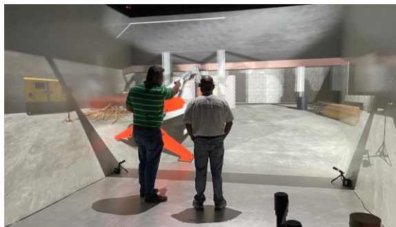
Figure 1. CAVE-type immersive display system used to present virtual reality environments and tasks in the NIOSH Virtual Reality Laboratory.
